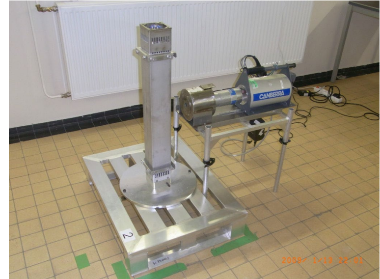
Nuclear material detection in MOX – mixed oxide fuel –fuel by using planar HPGe detector (MOL, Belgium)
