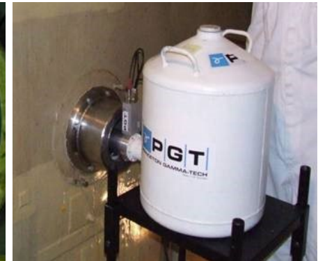
Spent fuel burnup characterization measurement using a coaxial HPGe detector and a narrow collimator (Paks NPP)
