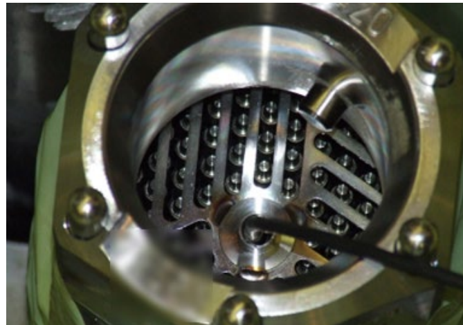
Verification of U-enrichment in fresh fuel assembly by using a CZT detector to measure inner pin enrichment (Paks NPP)
