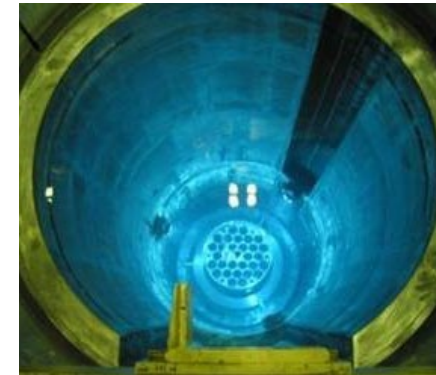
Spent fuel burnup characterization measurement using a coaxial HPGe detector and a narrow collimator (Paks NPP)
