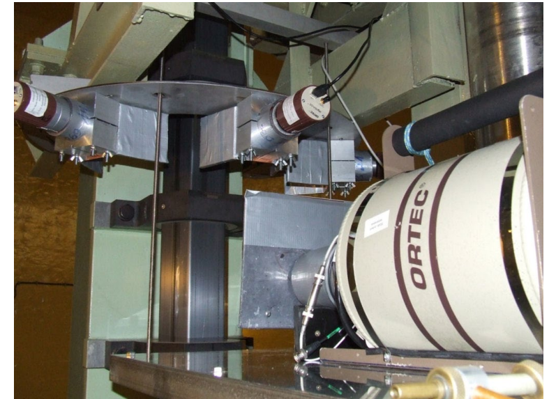
Verification of U-enrichment in fresh fuel assembly by using \text{LaBr}_3 (above) and HPGe (foreground) detectors (Paks NPP)
