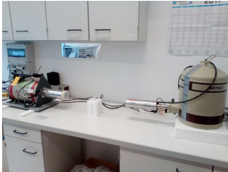
Measurement of a calibration source with 2 HPGe detectors (planar and coaxial) in the Gamma laboratory
