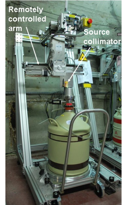
Facility from Gerda neutrino experiment
