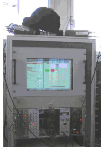
Beta-emitting nuclide measurements by liquid scintillation (TDCR)
