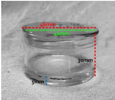
**Geometry 42mm diameter with data for calculating the energy/peak shape/efficiency**
