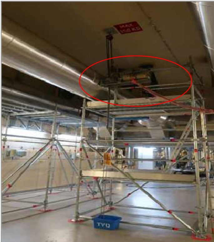
In-situ HPGe measurements from piping (2 m high) in Olkiluoto
