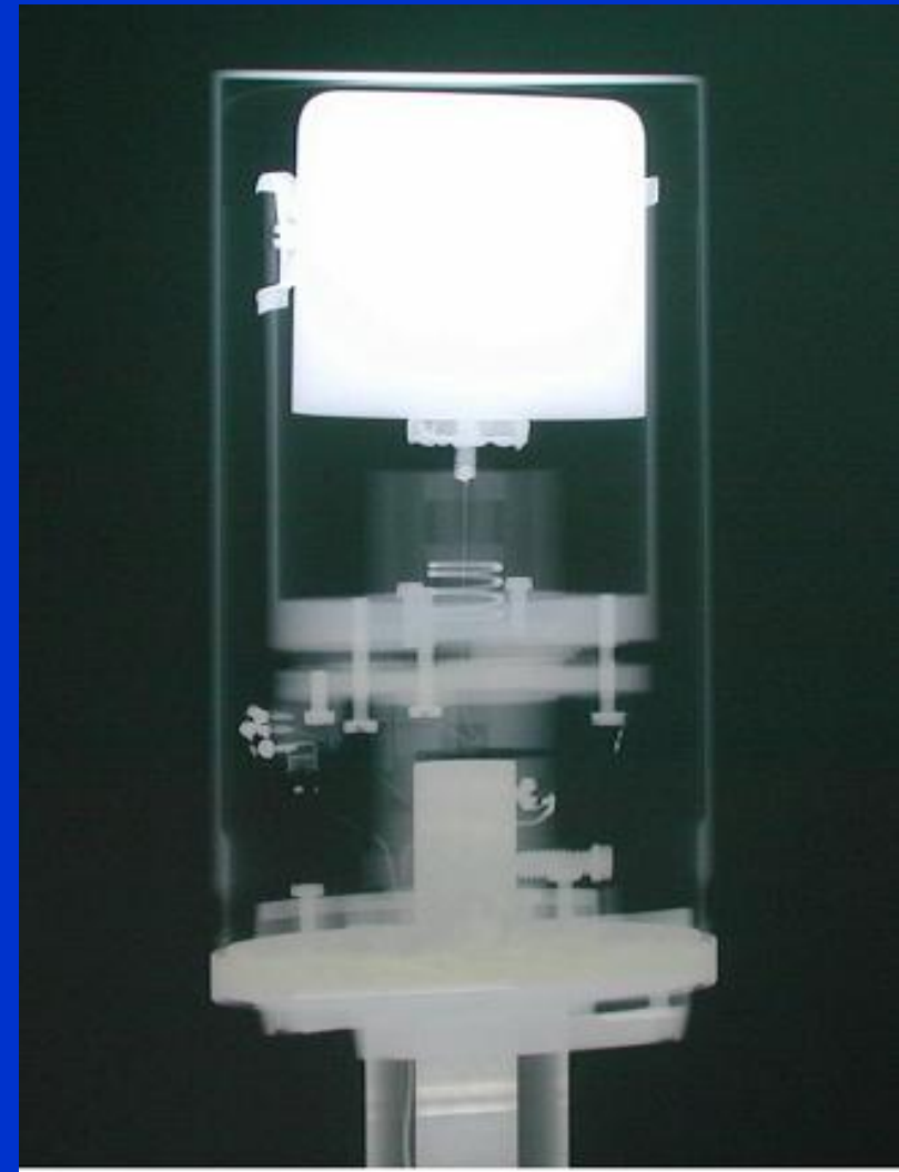
Radiography of a HPGe detector: Rounded crystal, axially shifted, tilted 2-10
