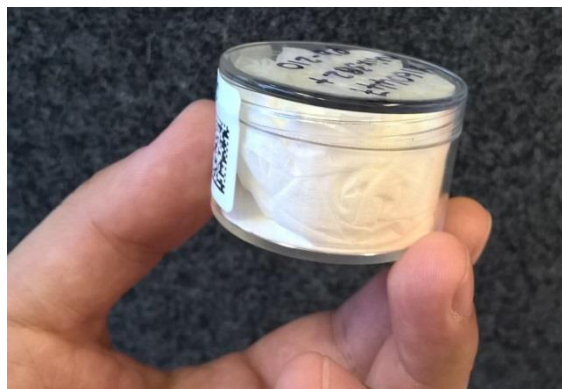
Beaker inner diameter 42 mm
