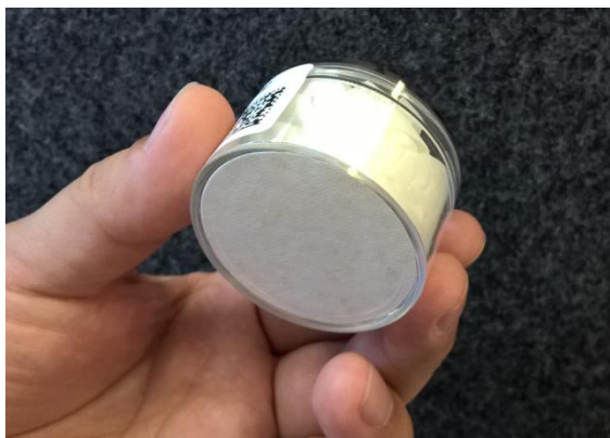
Beaker inner diameter 42 mm
