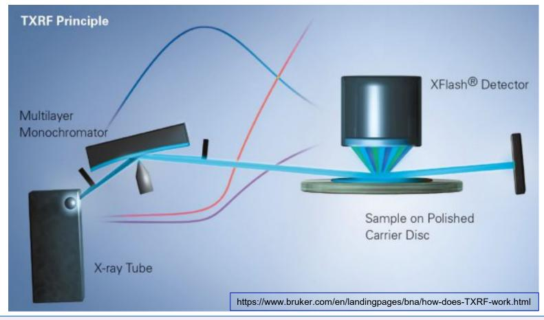
TXRF spectroscopy utilizes a multilayer monochromator to generate a fine beam which impinges on a sample at a very small angle for enhanced fluorescence yield and reduced noise enabling trace elemental analysis.
