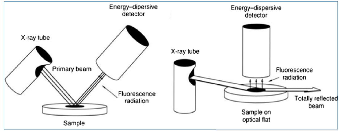
**Total Reflection X-Ray Fluorescence Spectroscopy** Tibo Yang, Xinyang Fan, Jinge Zhou Chengdu University of Technology, Chengdu, China.
