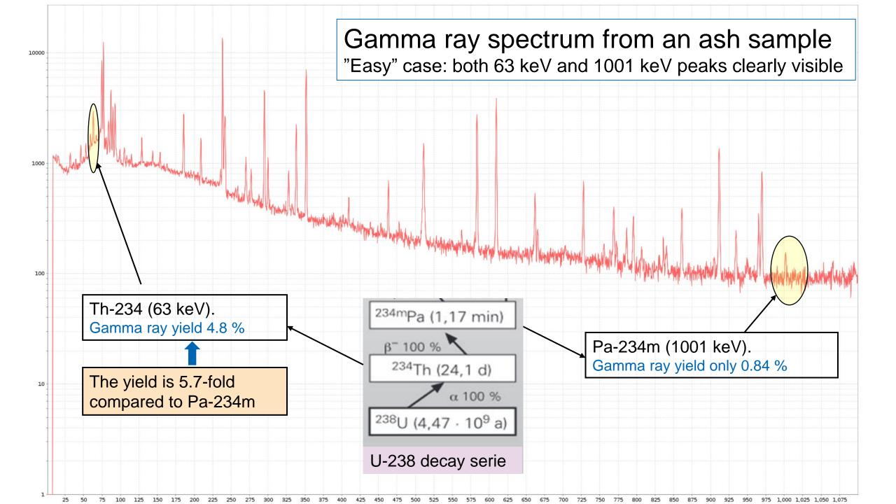
Comparison of peak efficiency between Th-234 (63 keV) and Pa-234m (1001 keV): At the energy of 63 keV the efficiency is by a factor of 6.2 higher than at the energy of 1001 keV.
