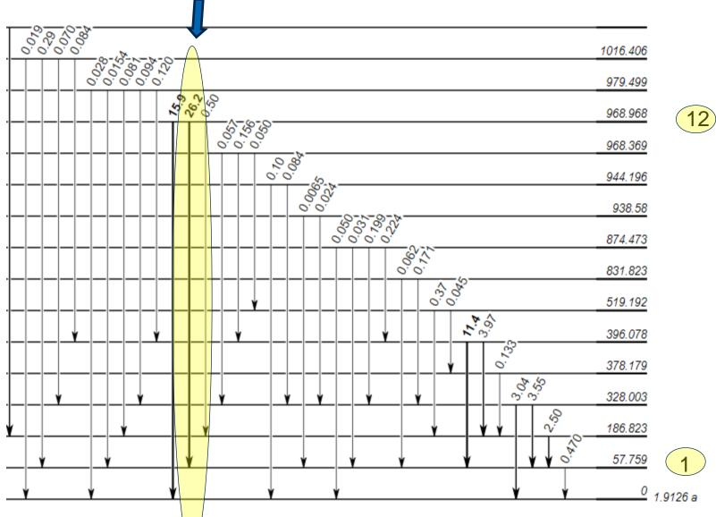
Transition from state 19 -> 12 has large K-conversion coefficient  $\alpha_k$ = 80 ja  $P_{\gamma+ce}$ = 5,5%.
