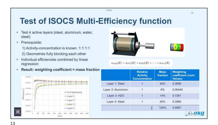
**Updated methodology with ISOCS Multi-Efficiency** Partial geometry 1: Beaker Template Partial geometry 2: Beaker Template 1. All activity in back tube bundle, All activity in front tube bundle, Back parts = passive absorbers, 2. Front parts = passive absorbers, geometry preserved geometry preserved Weighting coefficients = 0.10 Weighting coefficients = 0.90 Rel.Act. Rel. Act. Conc. Conc. 0.00 1.00 1.00 0.00 Detector Detector liloka **Comparison of methods**
