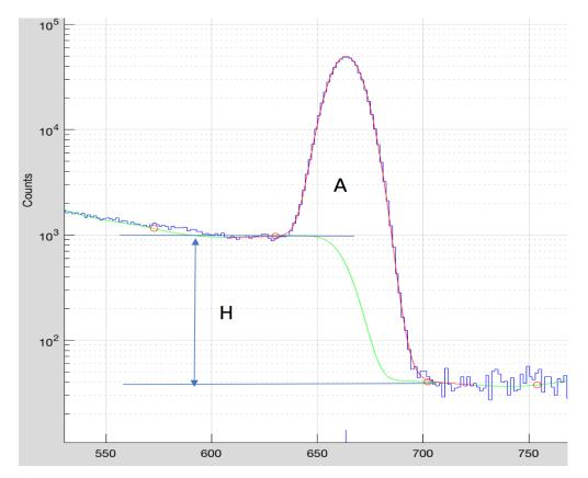
Cs-137 measured with RanidPro200 Backbag spectrometer
