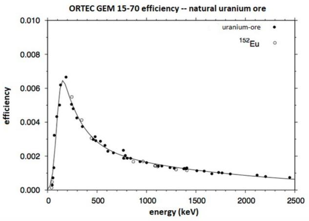
42 data points: <sup>234</sup>Th: 3, <sup>234m</sup>Pa: 2: <sup>234</sup>U:2, <sup>230</sup>Th: 1, <sup>226</sup>Ra: 1, <sup>214</sup>Pb: 5, <sup>214</sup>Bi: 14 efficiency-curve can be extended toward higher energies, up to 2447.9 keV (<sup>214</sup>Bi) without exact uranium-mass: relative efficiency curve: extended to absolute by an additional standard (<sup>152</sup>Eu)
