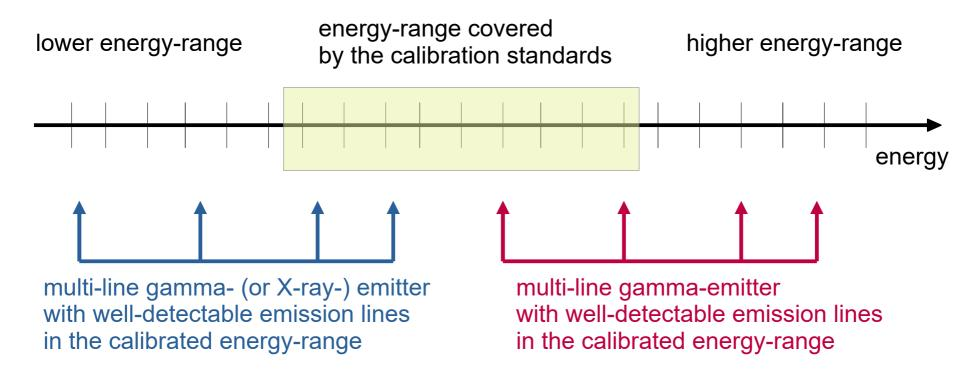
The sources used to extend energy-range should not be calibrated, only the indentical sample geometry is needed.
